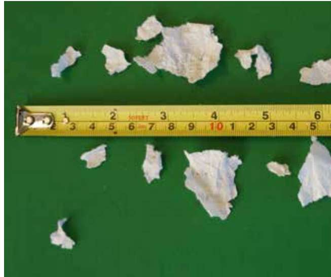
SHREDDER MAC 1500 D GRIDS 38 MM
