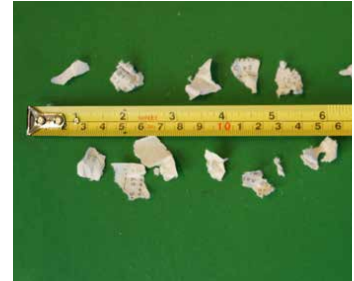
SHREDDER MAC 1500 D GRIDS 28MM
